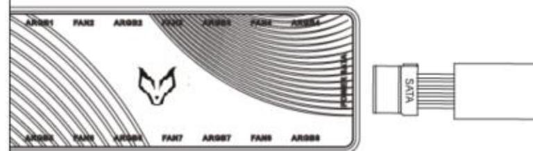
Connectez un câble SATA de l'alimentation au port POWER SATA du hub. *Connect the SATA terminal of the power supply to the Power SATA port on the hub.*
