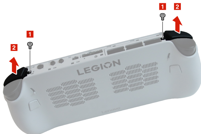
Figure 6. Remove screws and remove bumper buttons
