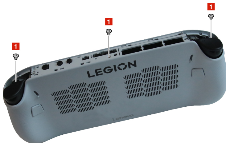
Figure 7. Remove screws at the top
