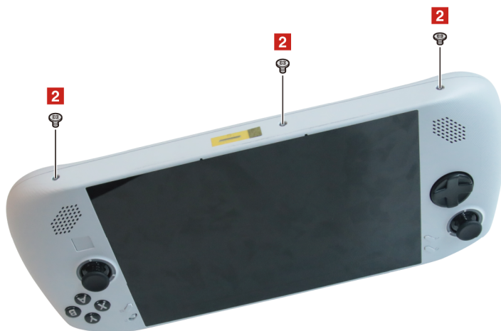
Figure 8. Remove screws at the bottom
