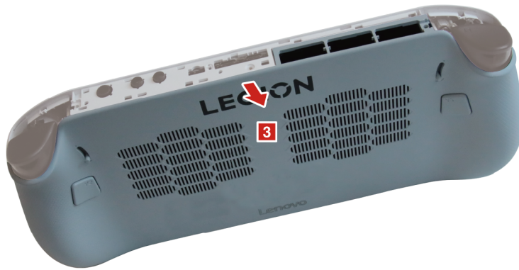
Figure 9. Remove the B cover
