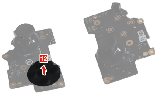
Figure 21. Remove the D-pad rubber
