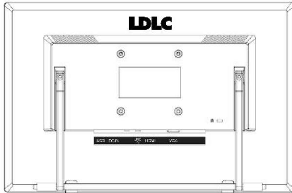
5. It is recommended to purchase a wall bracket that suits your device dimensions and weight. The wall support must also comply with the screen's VESA norm: VESA 75x75, 4 holes, M4, 8 mm, 8kg.
