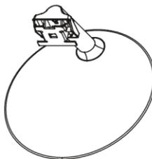
3. Place the top of the mounted base frame flat on the lower side slot of the rear case, adhered and push up, to insert the base stand into the rear case.
